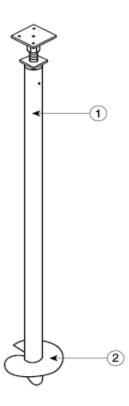
Figure 1. "Pro Post Foundation Screw Piles"
